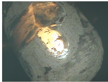
Flake of sulphur sulphide at tap changer contact
