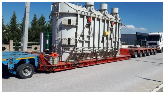
Road transportation of power transformer
