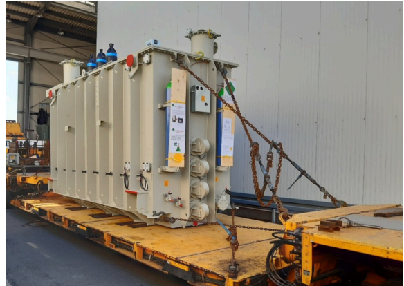
Transportation of partially assembled power
